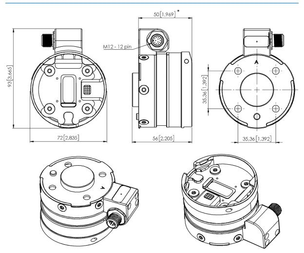
\* Distance from Robot flange interface to OnRobot tool All dimensions are in mm and [inches].
